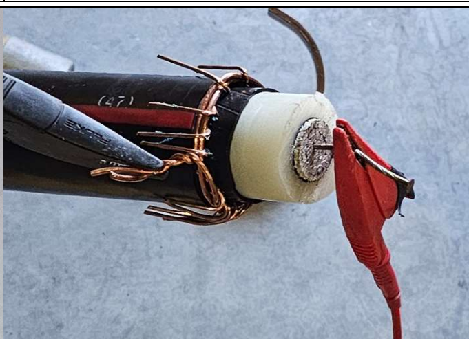
Figure 4: Concentric neutrals bound and test connections
